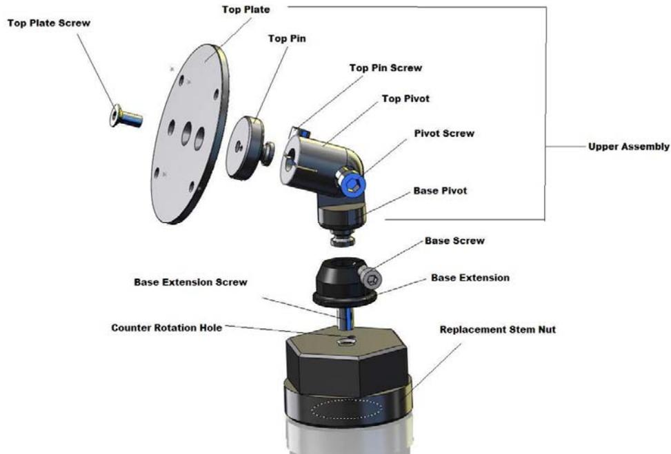
This mount system is designed to securely mount your device onto any Yamaha FJR 1300 by replacing the original stem nut. Please follow the installation instructions carefully. The mount is fully assembled and ready to install. The four (4) small holes in the top plate are the AMPs pattern found on many electronic accessories. The single 1/4" (6mm) hole is used for mounting cameras with thumb screw mounting holes.
